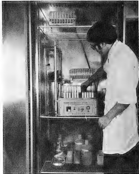
Figure 5.--Sephadex chromatography columns are kept in a cold incubator. Serum samples are separated by filtration through the gel column; fractions are collected and analyzed for specific antibody content.
